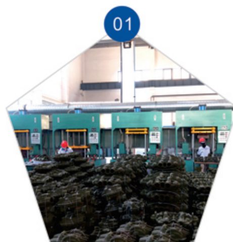
覆膜砂铸造制壳
